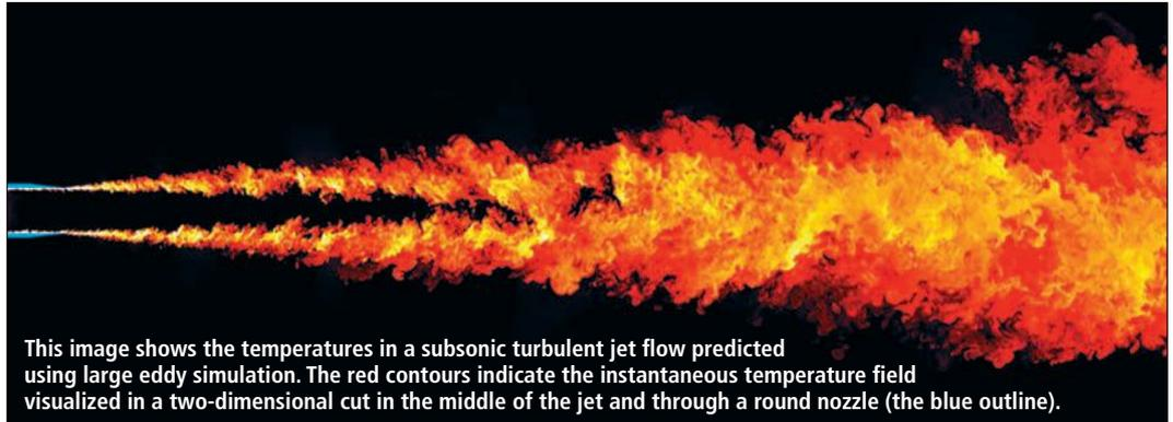
This image shows the temperatures in a subsonic turbulent jet flow predicted using large eddy simulation. The red contours indicate the instantaneous temperature field visualized in a two-dimensional cut in the middle of the jet and through a round nozzle (the blue outline).
