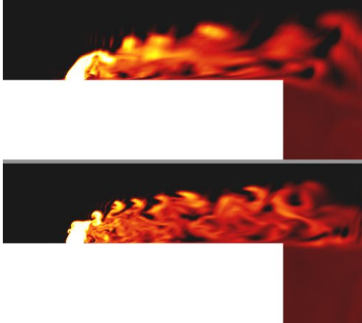
Figure 7. Comparison of mixture fraction for the two simulations with medium and locally refined grids. Contours are from 0 to 1. Top: medium size grid; bottom: locally refined grid. It is clear that the structures are more resolved in the locally refined grid.
